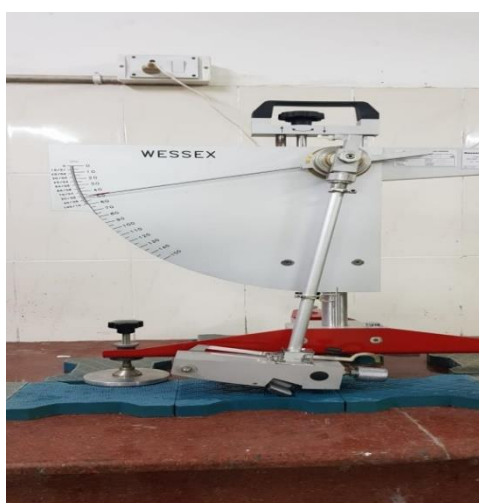
Figure 3: Skid resistance of composite tile by British Pendulum Tester
