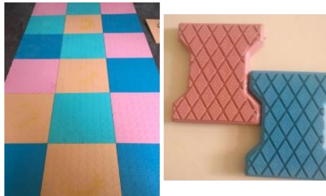
Figure 4: Interlock floor tiles and paver tiles made from waste plastic
