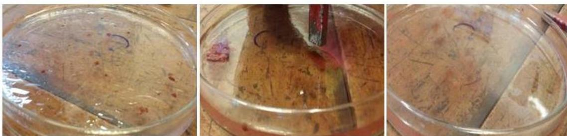
**Figure 4:** Extraction of lubricant oil from oil-water mixture using iron oxide nanoparticles
