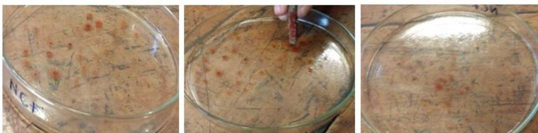
**Figure 3:** Extraction of mustard oil from oil-water mixture using iron oxide nanoparticles
