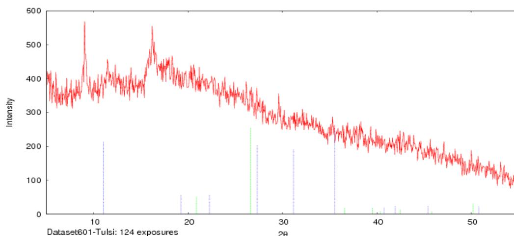
**Figure 2:** XRD spectra of synthesized CuNPs using Tulsi extract
