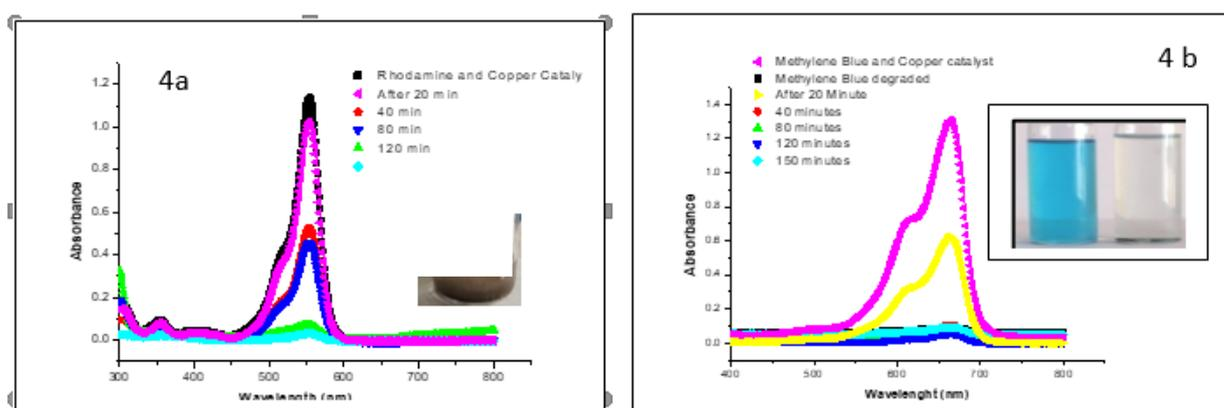
**Figure 4a:** UV-Visible spectrum of Rhodamine B dye degradation (Inset: complete degradation of Rhodamine Dye).
