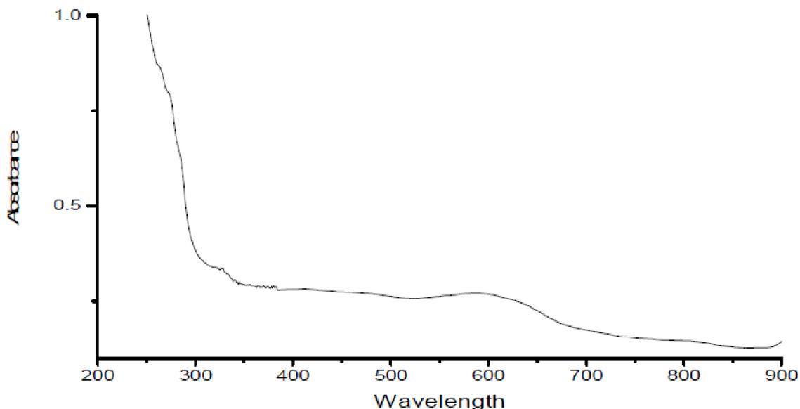
**Figure 1:** UV/Vis spectrum of as-synthesized CuNPs (a surface plasmon absorption band with maximum absorbance at 600 nm)
