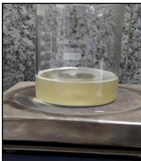
Figure 4: Aqueous Chitosan solution obtained after overnight stirring at room temperature
